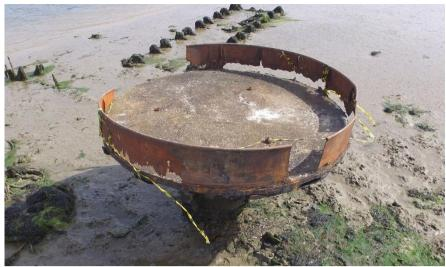
Figure 29: Fighting top showing fixings.
